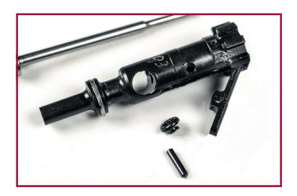
10. The Bolt is now disassembled.
