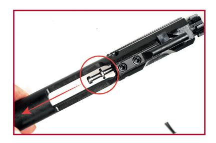
4. Push the Bolt back into the Bolt Carrier.
