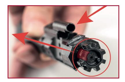
3. Insert the Cam Pin into the hole.
