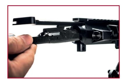
5. After removing the Bolt&Carrier Group completely, pull out the Charging Handle and tilt it downwards, proceeding with removal.
