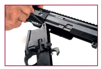
3. Insert the Charging Handle lever inside the Upper proceeding in an inclined direction, as shown in the photograph.
