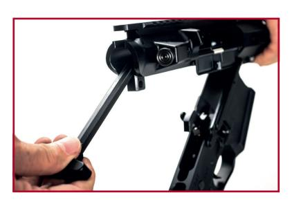
4. Insert the Bolt&Carrier Group inside the Upper (Bolt Carrier Key pointing towards the barrel).
