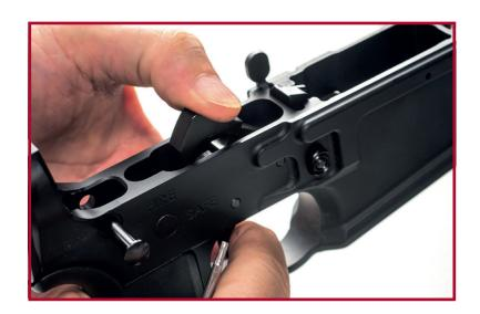
9. Ensure the hammer is in the cocked position and the safety is on.
