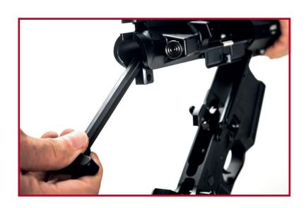
6. At this point we will have totally extracted the Bolt&Carrier Group and the Charging Handle.
