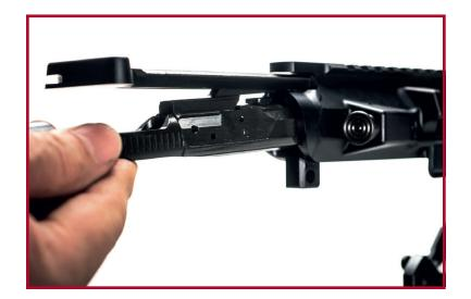
5. Complete the reassembly of the rifle by rotating the Lower until precise engagement with the Upper.
