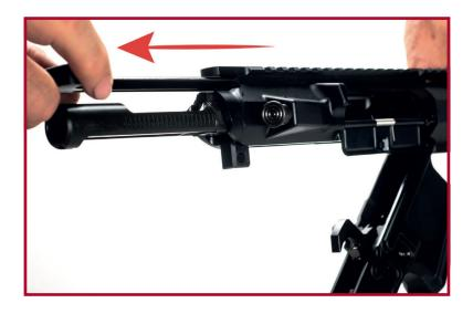
4. Pull the Bolt&Carrier Group to the rear and out of the back of the Upper receiver. Leave the charging handle. In case of bolt carrier with left or right charging system, remove first the "system" by disassembling the screw.
