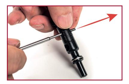
9. Lift out the extractor and spring. Do not remove the spring from the extractor. The extractor needs to be cleaned only when damaged or extremely dirty.
