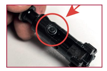
2. Place the extractor in its housing, making sure that the spring with "o-ring" engages correctly inside the cable clamp on the extractor.
