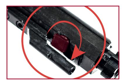
5. Insert the Firing Pin inside the Bolt Carrier.
