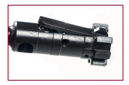
3. Pressing with the thumb the extractor (which mechanically will oppose a strong resistance, so if you could not manually make use of a clamp taking great care not to damage the parts) proceed with the reinsertion of the extractor pin. Eventually help yourself with a small rubber mallet.
