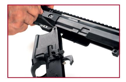
8. To proceed with the removal of the "Recoil Buffer", lower the "Hammer" to the correct position. Insert the safe.
